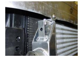
6/ Remove the horns from their brackets, now remove each bracket from the car and refit the horns as per the pictures below with the new brackets supplied so they are now sited higher. This is to allow the new hoses a free routing below the horns.
