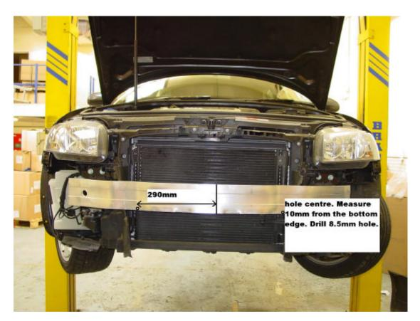
5/ Fit the brackets to the crash bar with the bolts/nuts supplied, fit the intercooler to these brackets as shown below. Tighten all the brackets and intercooler fixings once the intercooler is positioned centrally.
