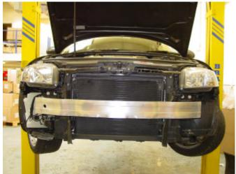
3/ Remove the 8x T25 screws in order to remove the complete engine under tray. Remove both lower standard intercooler hoses; these are just clipped in via a spring clip. Prize this away with a flat end screwdriver to aid removal of the hose end fitting, these will not be refitted but the seals are required later so place to one side for now.
