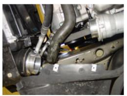
8/ Now fit the new hoses to join all the couplings and the new intercooler. The hoses may require a test fit to make sure they do not foul on any other engine or front panel components. A small amount of trimming may be required on the hoses at the new intercooler joints. Once you are satisfied with the fitment then secure all the hoses with the hose clips supplied.
