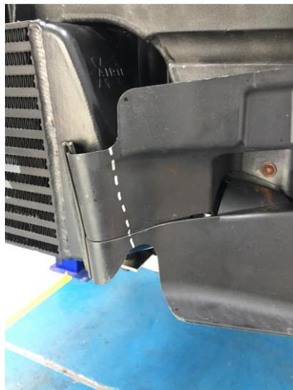
Remove the ambient air temp sensor bracket and bolt to modified crash bar with m5 x 16 socket head bolt and nylock supplied
