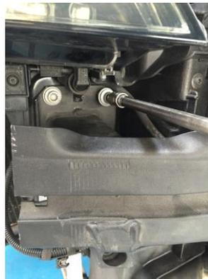
Once intercooler in place mark and drill holes, once happy bolt intercooler to modified crash bar
