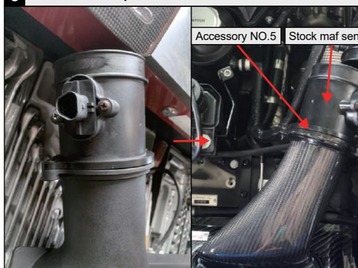
7 Place the carbon fiber tube to carbon fiber inbox and tight up with steel hose –no.13.
