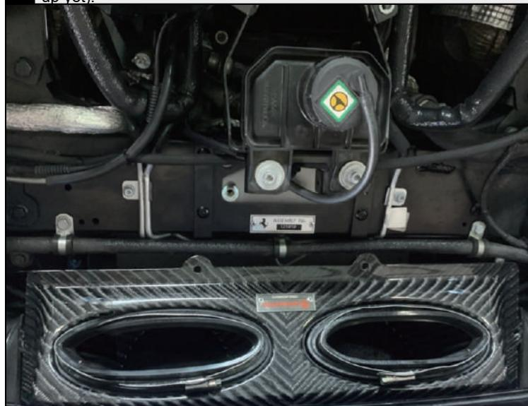
5 Install the stock maf sensor to the carbon fiber tube.
