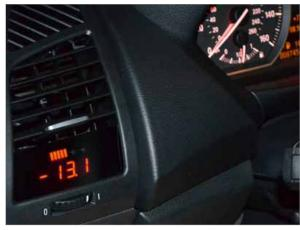
Start the engine and make sure the gauge turns on now that everything is hooked up properly, then fully re-install the vent and surrounding panels/trim.
