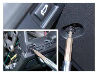
Remove the light switch panel by removing two #20 torx screws at the top, and one at the bottom as shown.
