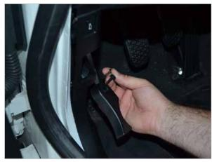
Replace the hood pop lever and then replace the footwell cover below the steering wheel.
