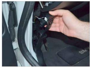
Flex this panel forward to get access to the OBD2 port and the trunk pop switch. You will need to pull the rubber door seal forward to free the panel.
