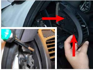
There are 2 SQUARE holes in the dash left of the vent, these holes allow you to press the vent's tabs through the holes to release the vent from the dash.
