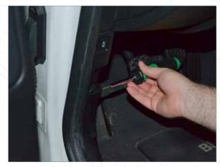
Remove the side kick panel cover screws, first remove the Phillips screw holding the hood pop lever, then the screw behind the lever. 2 screws total.
