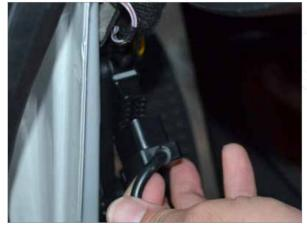
Plug in the obd2 connector to the car.
