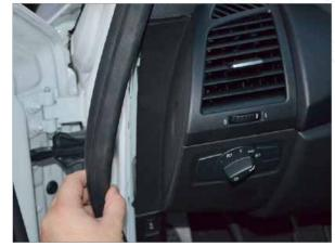
With the driver's door open, pull off the rubber door seal, it is just a friction fit.
