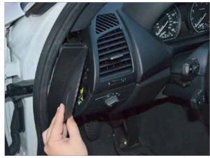
Remove the side dash cover as shown. It is easiest to start at the bottom of the panel first.
