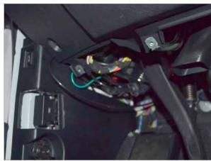
Replace the side kick panel and tuck/secure the control box and harness up above this panel near the other factory
