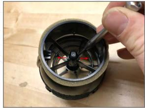
Use a screwdriver to spread tabs and release center shaft as shown
