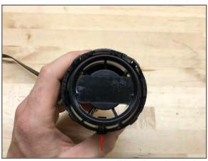
Seat display in vent housing (slot shown should in 6 O'clock position when installed in vehicle)
