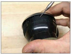
Release three remaining tabs under felt at 3, 9, and 12 O'clock positions
