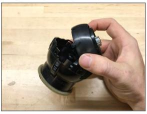
Remove slat assembly from housing
