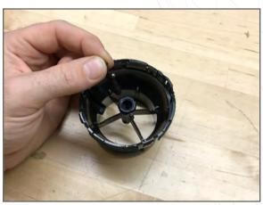
Remove center shaft from front of housing
