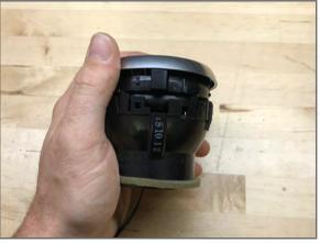
Reinstall trim ring onto vent housing
