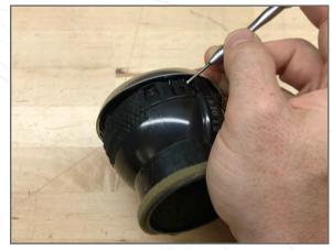
Using a small screwdriver release the tab on the bottom of the vent (6 O'clock position)
