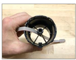
Feed display cable through housing as shown
