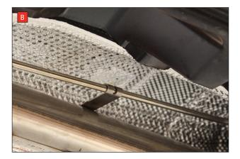
A) When Fitting the GPF delete pipe the original system requires cutting 80mm from the centre mounting bracket. De-bur this edge as the Scorpion adaptor will fit over it.
