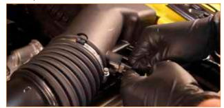
**05.** Loosen the worm-gear clamp that secures the induction pipe to the airbox, and separate the induction pipe from the airbox.
