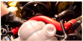
Compress the spring clamps that secure the lower radiator hose to the vehicle and slide them down the hose, out of the way. Then remove the lower radiator hose from the vehicle.
