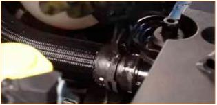
**09.** Slip two worm-gear clamps over the Mishimoto upper radiator hose and install it on the vehicle. Secure the hose to the radiator and water outlet with the worm-gear clamps. (2x worm-gear clamps)
