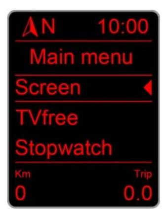
In the top of the screen is always signalized the menu name, in this example, you can read Main menu, this means we are in the main screen of the PolarFIS configuration menu. The main menu screen has the next options:
