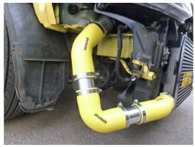
16. Re-fit crash bar and Install Intercooler alloy spacer tubes as shown below & tighten Intercooler fully
