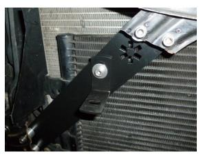
14. Bolt Intercooler to Top brackets 'Loosely'
