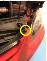
3. Undo 2x plastic screw fittings holding inner arch to bumper and 3x 8mm bolts underneath
