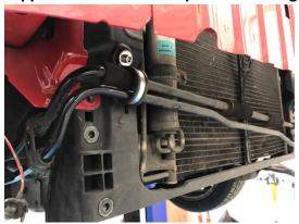
13. Loosely fit intercooler into place and secure with supplied M6 x 20 socket head bolts and washers
