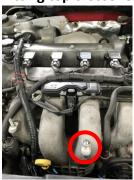
Fit 90 degree silicon reducer from turbo to crossover
