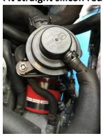
Fit hard pipe with BOV outlet into silicon then 90 degree silicon connects into intercooler
