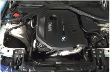
Secure the hose coupler on both end with clamps following 3 the prefer torque setting.
