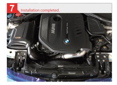
When fastening the metal hose clamp, recommend set tightening torque at 1.5Nm.Otherwise, it might result in deformation or crack if overtightening.
