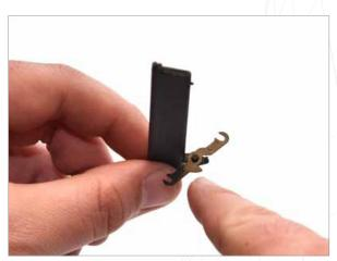
Now remove the second from bottom slat, this slat will have a small metal controller bar behind it that will need to unhook from the slat above it as it comes out. Once again, take care that the other slats do not come out.
