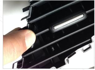
Place index finger over the central control slat while removing lower slats. This will insure control and upper slats remain in the vent and in union with one another.
