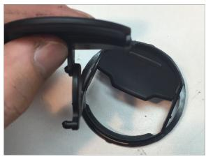
Remove lower vent slat and bracket.
