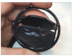
Install display into vent slat bracket. NOTE: Display glass goes behind lip at bottom of bracket.
