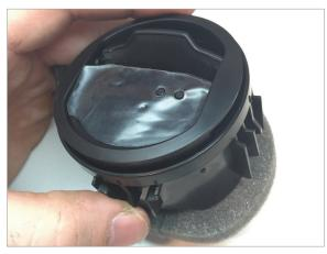
Snap black trim ring onto bracket and install into vent barrel.
