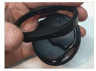
Take vent slat bracket out of barrel and remove black trim ring.
