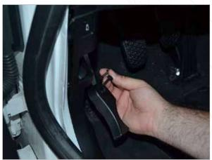
Replace the hood pop lever and then replace the footwell cover below the steering wheel.
