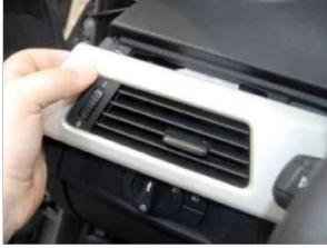
With the driver's door open, remove the vent from the car with trim attached.
