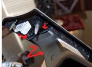
Unclip the vent from the trim; release it from the clips on one side and bottom, then pull away to release the other side.
