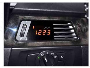
Start the engine and make sure the gauge turns on now that everything is hooked up properly, then fully re-install the vent and surrounding panels/trim.
