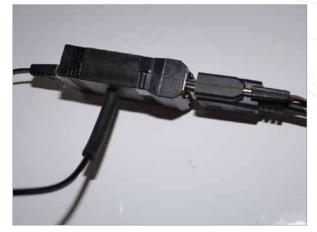
Connect the vacuum line and harness to the control box as shown. (note: for versions earlier than 2.1, the vacuum port is on the harness)
