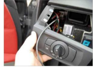
Remove the light switch assembly to give yourself room to work, it just pulls out.
