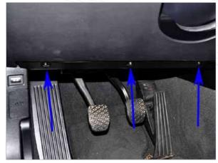
Remove the lower dash cover below the steering wheel by removing the three #20 torx screws shown here. Lay this cover down into the footwell.
