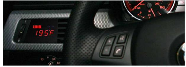
Enter the config menu for the gauge. See the config details at <a href="https://www.p3cars.com/install">www.p3cars.com/install</a> Configure your engine type. Calibrate the boost sensor to your ambient pressure.
