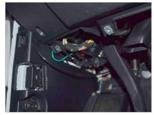
Replace the side kick panel and tuck/secure the control box and harness up above this panel near the other factory wiring.
