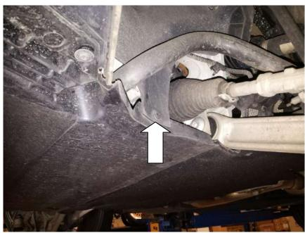
6. Using a T25 Torx driver remove 3x screws inside the edge of the arch liner and 2x T25 behind the wheel on both sides of the vehicle.
