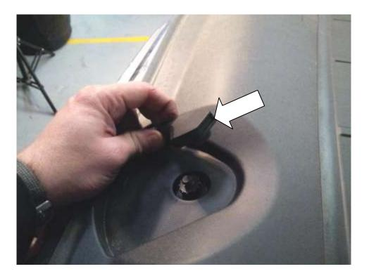
4. Starting on the front edge carefully pull the plastic cover upwards to release it, then slide the panel forwards to remove it.
