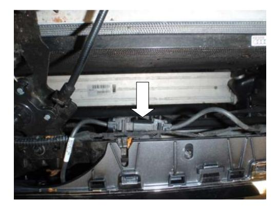
1. Using a T30 Torx, extension short bar and suitable small ratchet (ideally ¼" drive) undo 1x bolt located underneath headlight on the inside of the wing on both sides. This is very awkward, as you cannot see the bolt you are trying to undo.
