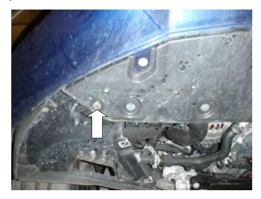
9. Carefully pull the arch liner to one side. Using a panel-clip removal tool or flat blade screwdriver remove the vertical plastic clip, if necessary lubricate the plastic clip with silicone spray or similar.
