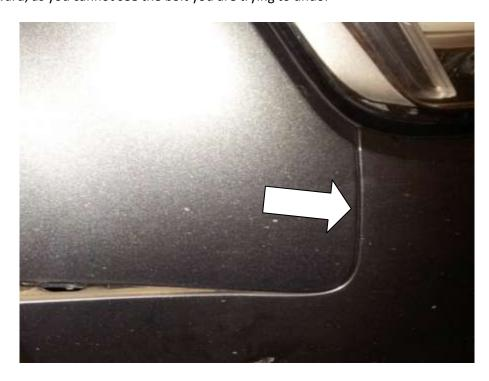
13. The next part requires two people. Carefully pull the bumper away from its mounts starting at each wheel arch. If one person supports the weight of the bumper the other can reach inside and disconnect the large electrical connector on the left-hand side of the vehicle.
