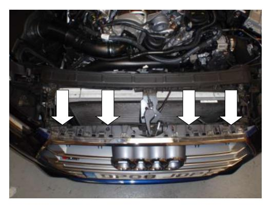
12. Disconnect the wiring to the bumper-mounted sensor and unclip the sensor-mounting bracket.
