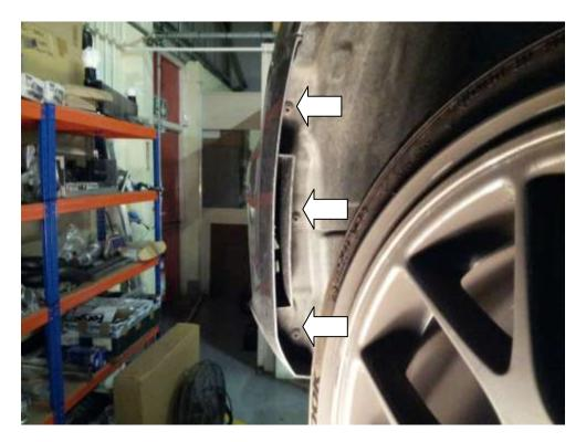
7. Using a T30 Torx driver undo 5x screws.
