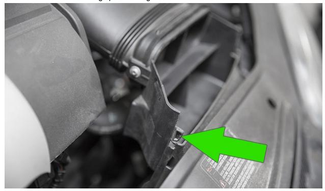
**4.** Unplug the mass air flow (MAF) sensor and place safely out of the way..
