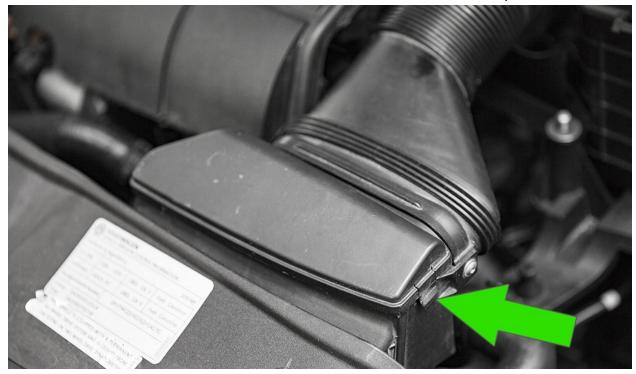
**3.** The air inlet is comprised of two parts, one section on the radiator support and another section of the air inlet on the engine cover. Separate these two halves by depressing the plastic tabs on both sides while lifting up on the engine cover side inlet section.
