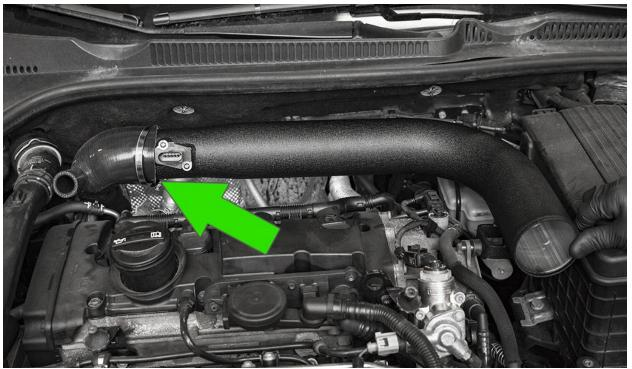
**14.** With the intake pipe in place, install the rubber isolator stud through the vacuum pump on the side of the cylinder head. Install with the supplied washer and 10mm nut and tighten by hand.
