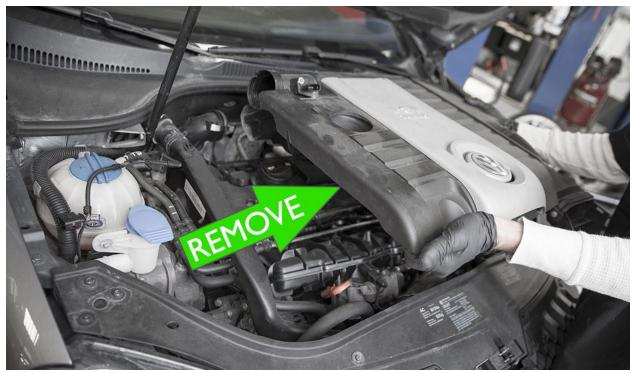
**7.** With the engine cover out of the way, you will now remove the final section of the air inlet mounted to the radiator support. Remove the two mounting screws with a T25 torx driver.
