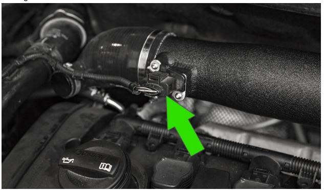
**24.** Align silicone turbo inlet, silicone hump coupler, and intake pipe positions so everything sits in place straight, relaxed, and without tension. With the complete intake assembly properly positioned, tighten all four hose clamps firmly.
