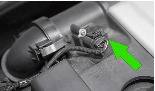
**5.** Using a flat head screwdriver, release both clamps on the turbo inlet pipe and pull back to release the o ring sealed inlet from the engine cover..
