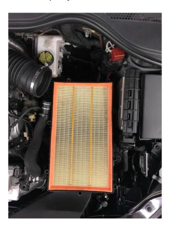
Step 9 – Remove the factory panel air filter from the lower air box.
