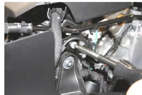
9. Remove T30 Torx screw from metal support bracket on side of engine just below engine cover.
