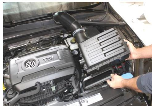
4. Lift out factory air filter box from its (3) rubber grommet mounts.
