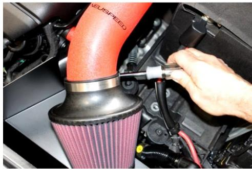
14. Adjust filter to have at least a 1/2" clearance above heat shield, and then tighten with 8mm nut driver.
