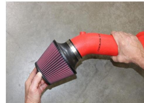
11. First loosely install NEUSPEED air filter onto intake pipe.
