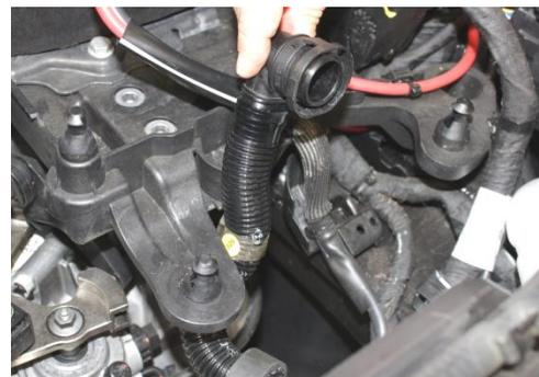
6. **AIR PUMP ONLY:** Pivot air pump hose to sit between the two front air box mounts.
