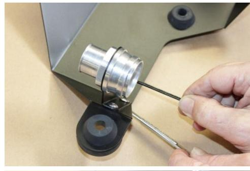
5. **AIR PUMP ONLY:** Mount billet air pump fitting with bracket to heat shield using supplied M5x8mm and lock nuts. Tighten with 3mm hex key wrench and 8mm wrench. Then install mini filter.
