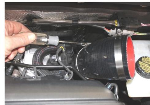
8. Install reduced end of 45° silicone hose with #44 SS hose clamp onto turbo inlet, position hose so that opening is pointing directly toward left side of vehicle, then tighten clamp.
