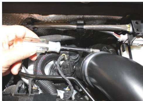
1. Disconnect air intake hose at turbo inlet using 7mm nut driver.
