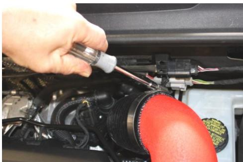
13. Tighten #48 SS hose clamp at intake pipe using 8mm nut driver.
