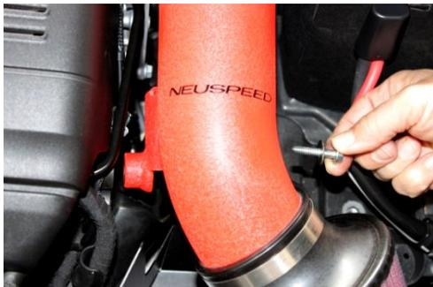
12. With #48 SS hose clamp loosely on silicone hose install *NEUSPEED* intake pipe, push on all the way until silicone hose meets bend in pipe. Then using supplied M6x30mm bolt attach pipe to rubber isolator and tighten.
