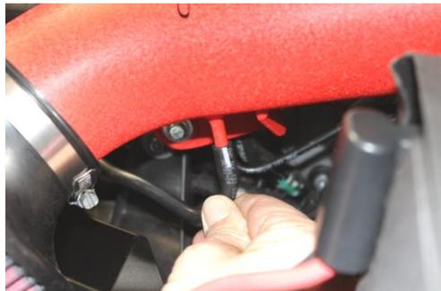
15. Connect vent line to *NEUSPEED* intake pipe.
