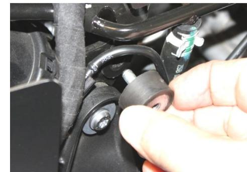
10. Install and hand tighten rubber isolator into threaded hole.
