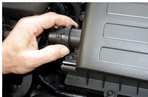
3. **AIR PUMP ONLY:** Squeeze collar to unlock and disconnect air pump hose from air filter box lid.
