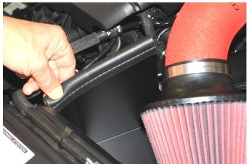
16. Install rubber strip on top-edge of P-Flo bracket.
