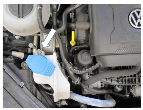
4. Attach the Forge lower bracket to the Forge washer bottle using 2x M4 x 6 (shorter) bolts supplied. Then screw the Forge tube to the bottle.
