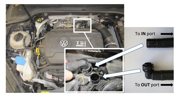
9. Once the hoses are neatly routed, attach supplied dual hose clamp and finally tighten bolts from Step 7. If you have fitted FMCTMK7WB then top up the screen wash fluid until visible in Forge bottle.
