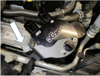
8. Disconnect the connector – squeeze plastic ring and lift. Attach hose ends as illustrated below
