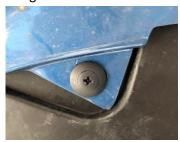
5. On top of the slam panel where the torx fittings were there is a plastic clip, this needs to be pushed up to release the clip and allow the top of the bumper to come forward, then using a second person starting from the edges of the bumper pull outwards to release the corners, unplug the wiring for the fog lights and then proceed to remove the bumper by pulling it out forwards and then store the bumper safely.
