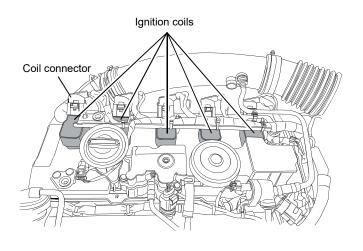
6 Install the Plasma Directs to the engine, and connect the coil connectors. Then, tighten the fixing nuts.
