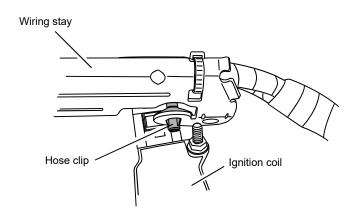
Remove the coil fixing nuts, and disconnect the coil connectors. Then, remove the ignition coils from the engine.
