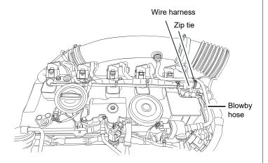
10 Place the engine cover back onto the engine.
