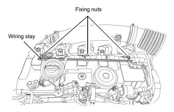
4 Remove the hose clip from the wiring stay. (The hose clip will not be used. Keep it at hand.)
